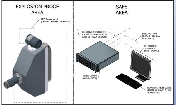
CAT6 Ethernet, however, has a distance limitation of 100m before there is signal loss that can interrupt analysis. In those situations, it is possible to convert the CAT6 Ethernet to fiber via CANTY's media converters. Refer to document TA11950-1024. Using this method, it is possible to run a fiber line up to 10km between the analyzer's power supply and then VCM. In this case, a typical layout of the components will look like the following.
