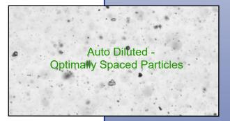
CANTY's Auto-Dilution System meters in known quantities of diluent based on the images acquired by the camera system. When there is extra space between particles, the software will lower the diluent flowrate. Conversely, if the image becomes too crowded, the software increases the diluent flowrate. By knowing the amount of dilution fluid added, if any, the concentration of particle before the auto dilution can be computed by the CantyVision Software and output to the end users control system.
