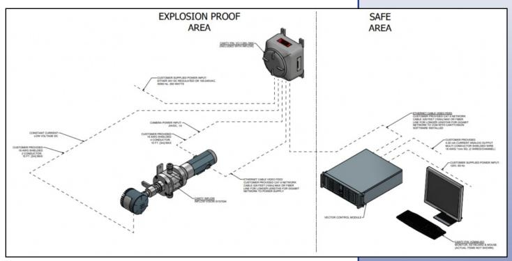
CAT6 Ethernet, however, has a distance limitation of 100m before there is signal loss that can interrupt analysis. In those situations, it is possible to convert the CAT6 Ethernet to fiber via CANTY's media converters. Refer to document TA11950-1024. Using this method, it is possible to run a fiber line up to 10km between the analyzer's power supply and then VCM. In this case, a typical layout of the components will look like the following.
