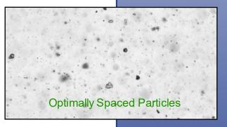
Using only a back light allows for a grayscale images to be obtained. Using a front allows a color image to be obtained where specs and the color distribution of the sample can be measured.
