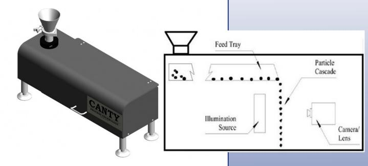
Given that the speed of the feeder can be controlled based on the number of particles seen on the image, overlapping particles on the image can be avoided allowing each particle to be independently measured for particle size, shape, and color while also allowing analysis to occurring as quickly as possible.
